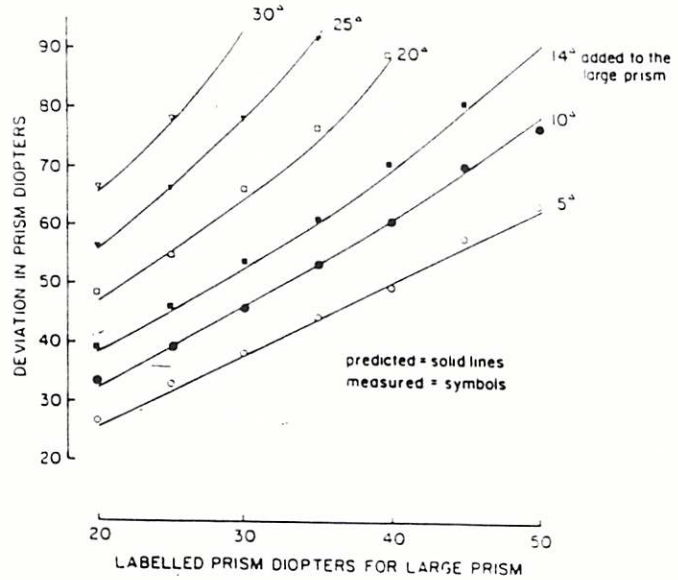
Fig 9. The deviation in prism diopters produced by adding a 5, 10, 14, 20, 25, or 30 Δ plastic prism to a 20, 30, 40, or 50 Δ plastic prism in the frontal plane position.
