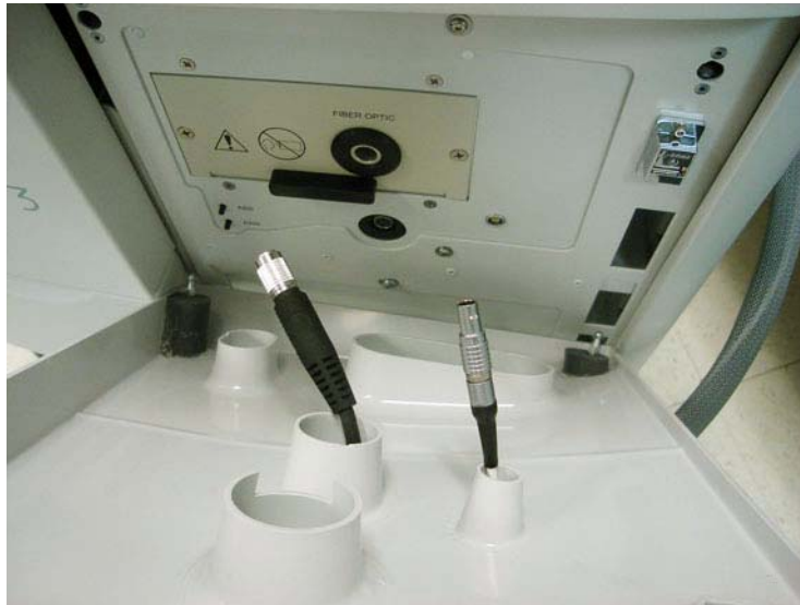
Figure 25 Threading cables through the front cover
