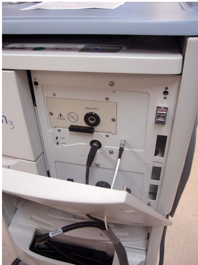
Figure 12 Light box cover removed
