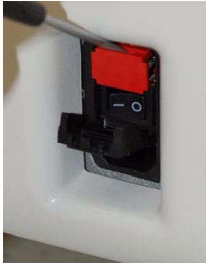
Figure 19 Fuse holder re-inserted
